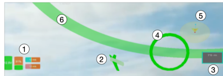
Figure 5: View from the security pilot with "Where is My Drone" second prototype. 1) to 4) as in Figure 4, 5) Radar view with the drone and pilot positions, 6) Line representing the current flight path.
