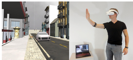
Figure 2: Person interacting with automated vehicles in a VR Simulation - interacting with an automated vehicle to indicate it should give way.
