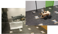
Figure 4: SLAM supplemented with tags
