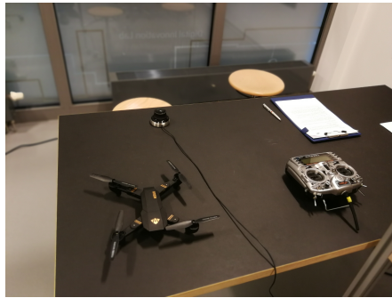
Figure 5: Study setup. During the study, the participant sat in front of the 3-D mouse and had to control a simulated flight.
