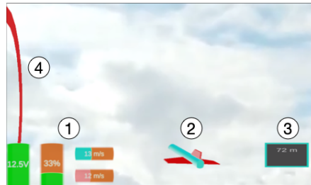
Figure 4: View from the security pilot with "Where is My Drone". 1) Gauges indicating the power and battery level, the air speed and the ground speed. 2) 3D model displaying the drone attitude 3) Drone's altitude and climb gradient. 4) The localization ring that helps finding the drone.
