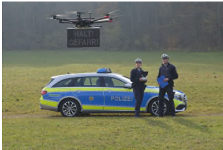
Figure 1: Police officers are using DisplayDrone to deploy a temporarily available “danger” sign that notifies passers-by about an upcoming hazard. The text on the display means “Stop! Danger!”
