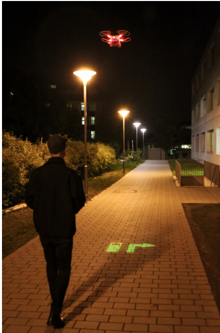
Figure 2: A pedestrian receives navigational instructions by a projector attached to a drone.
