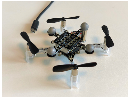
Figure 2: Our Crazyflie drone with MoCap marker deck and markers installed; Micro-USB connector used to charge the drone is in the background, for scale.
