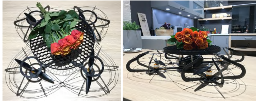
Figure 2: The design of our TrayDrone uses a tray that is designed after an air permeable honeycomb design. Further it comes with designed protectors for protecting the users and the environment from the drone's blades.
