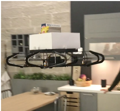
Figure 1: TrayDrone is carrying a box to be delivered to the user in a smart kitchen environment.
