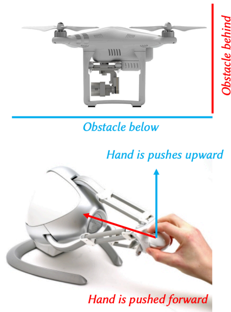
Figure 2. Example of use of kinesthetic haptic feedback to increase spatial awareness during the teleoperation of drones
