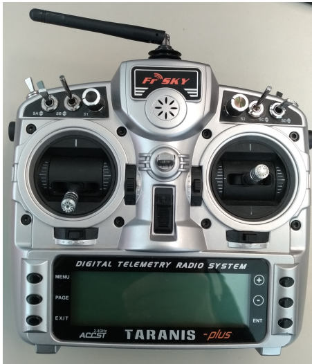
Figure 1: Currently, most non-autonomous drones are controlled by more or less complex remote control transmitters (RCT). The image shows one of the complex models.
